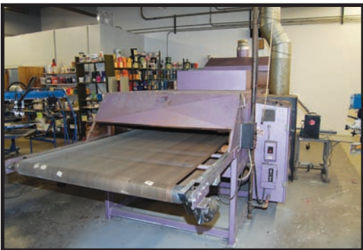
NATIONAL Gas Conveyor Dryer
