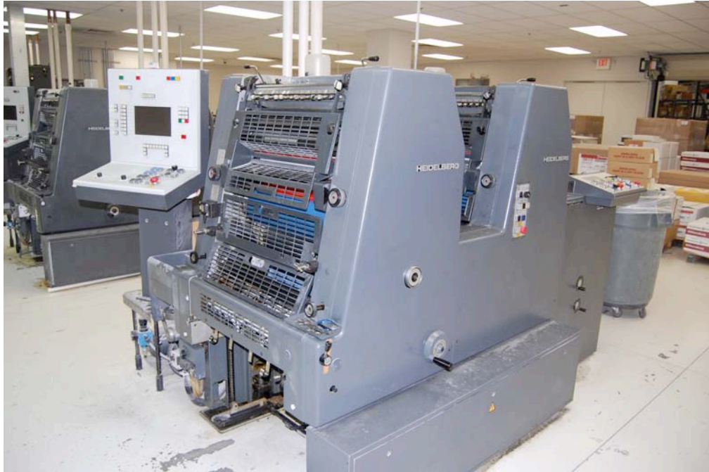
(1) Heidelberg, Model #GTPZPS-52, 2-Color Offset Press, s/n 708647, 47,721,503 Impressions, Kompacs Dampeners, Sheet Size 14.125" x 20.5", Stream Feeders, Perfector
