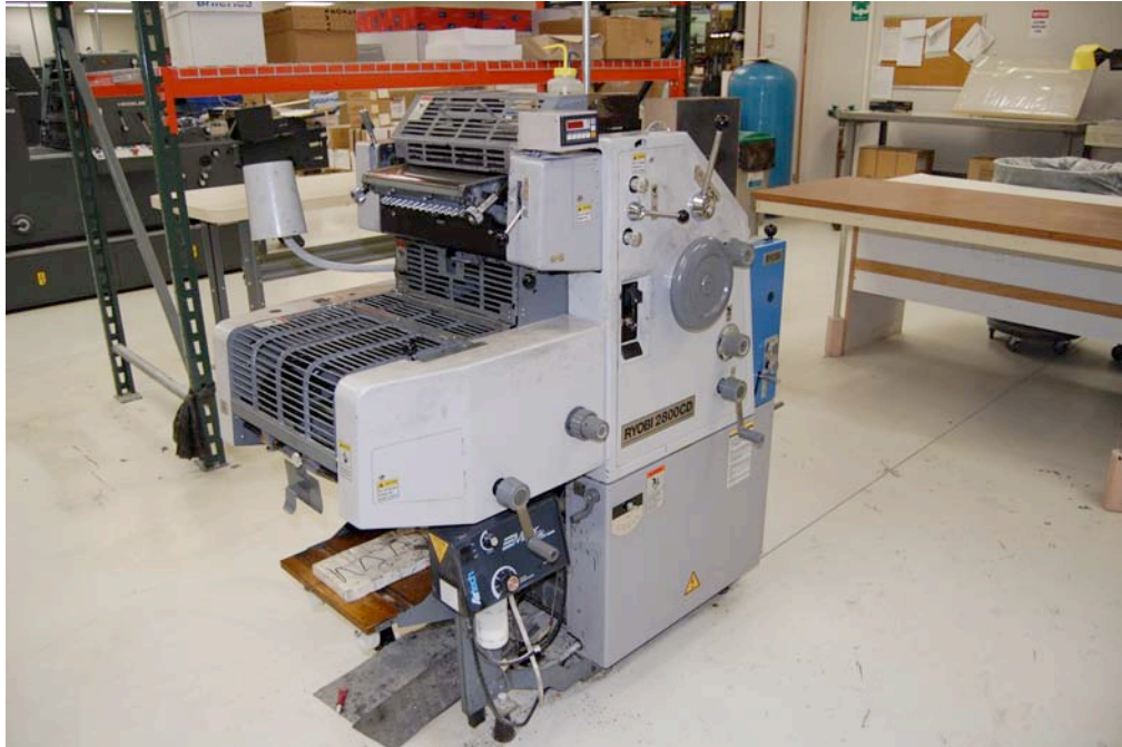
(1) Ryobi, Model #2800CD, 1-Color Press, s/n 19282, Impressions NA, Sheet Size, 12" x 17"
