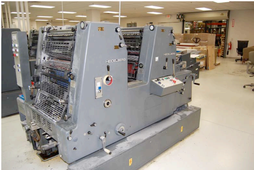
(1) Heidelberg, Model #GTOZ-52, 2-Color Offset Press, s/n 692349, 54,683,683 Impressions, Kompacs Dampeners, Sheet Size 14.125" x 20.5"
