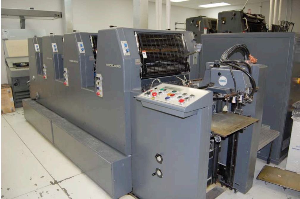
Heidelberg, Model #GTOV-S52, 4-Color Offset Press, s/n 705192, 82,936,288 Impressions, Kompacs Dampeners, Sheet Size 14.125" x 20.5", Stream Feeders
