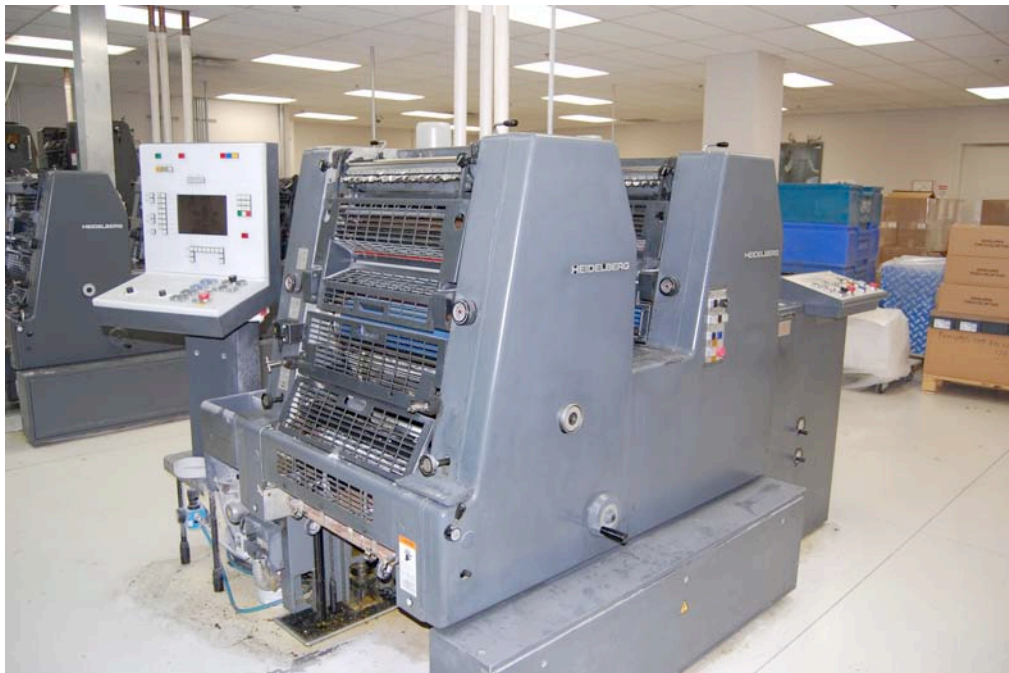
Heidelberg, Model #GTOZ-S52, 2-Color Offset Press, s/n 710262, 42,894,550 Impressions, Kompacs Dampeners, Sheet Size 14.1215" x 20.5", Stream Feeders
